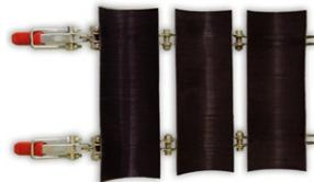
The coupling is to be opened to her full extend. The rubber coating dont be loose or damaged.
