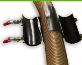
The anti slide mat has to be put around the hose formlockingly. The formation of wrinkles has to be avoided.
