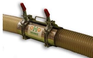
Fold in both outer shells and close the coupling with the force about 200 kN until the security lock snaps into place.
